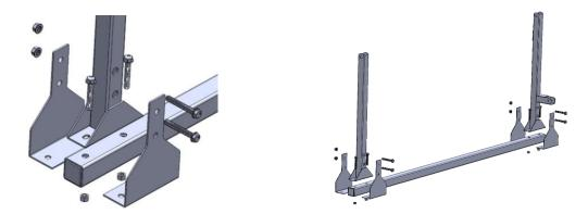
2. As you assemble, you will need to overlap and line up the 2 reinforcing plate holes (see label on the parts). Fully tighten these bolts and torque all bolts to min of 110 ft. lbs.
