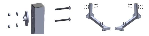
2. Install the left and right U channel brackets onto the arrow board using supplied long bolts, washers on both sides, and lock nuts. Make sure the tab on bottom is on the back side of the board. This is a safety stop to prevent board from falling forward into a windshield.
