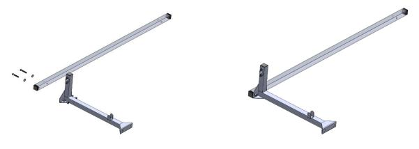
4. Slip the arrow board assembly onto the left "L" bracket, using two washers between the arrow board bracket and the "L" bracket to make room for rotation of the board.
